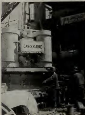
The new postwar Cargocaire dehumidifying unit weighing 50 per cent less, occupying only 1/2 the usual deck space, recently announced to the trade.
